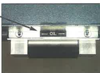
Oil bottom and top roller bearings with supplied Zoom Spout oil as shown.
