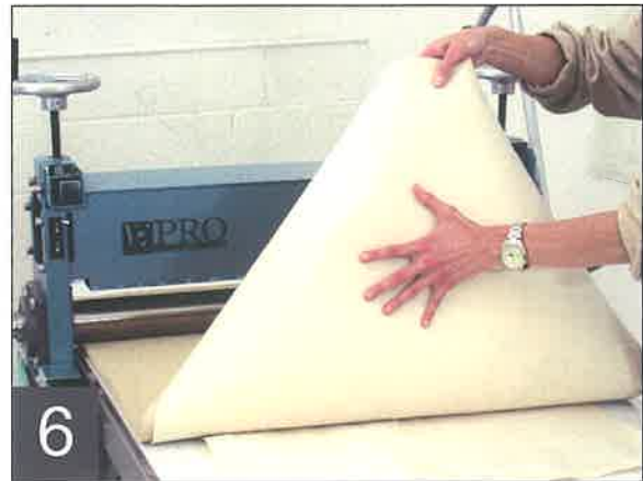
Place blankets and remove any wrinkles. Set pressure using the Pressure Gauges only.
