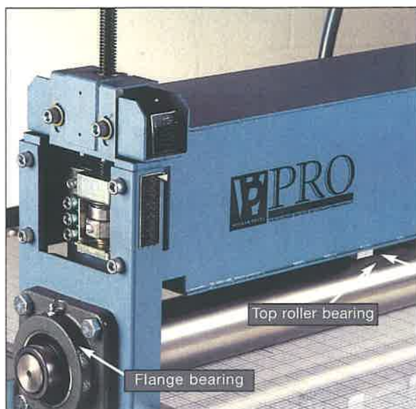
Oil bottom and top roller bearings with supplied Zoom Spout oil as shown.
