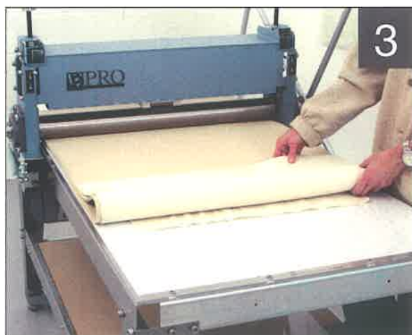
3 Trap the paper and the newsprint by advancing the print roller over the paper edge. Pull back the paper and blankets and lay over the beam.
