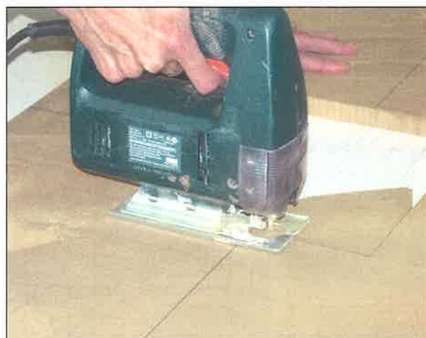
Cut the template along the outside of your plate line.
