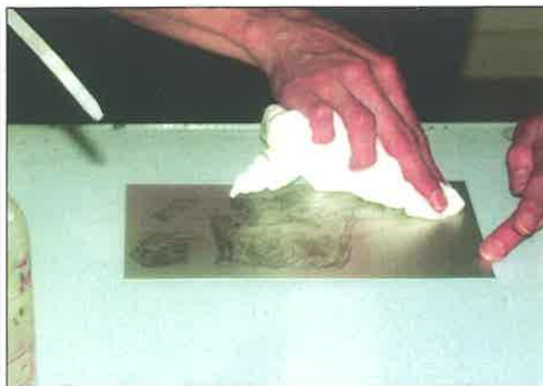
If necessary you can use denatured alcohol to remove any silicone not re-moved with water.
