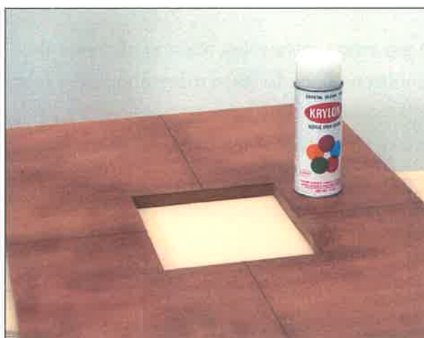
Seal the template with any sealer, we used Krylon Clear Spray Lacquer. Always spray out doors and wear a ventilator.
