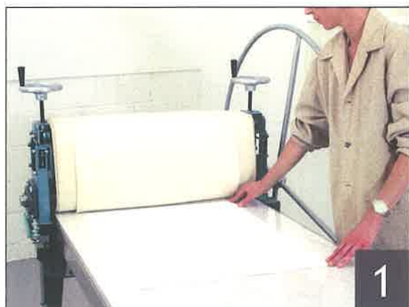
1 Lay the print paper face down and align to the paper corners on the grid.
