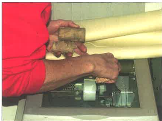
Carefully place objects on scanner bed. Glass top is easily scratched and once scratched will affect the quality of your scans.
