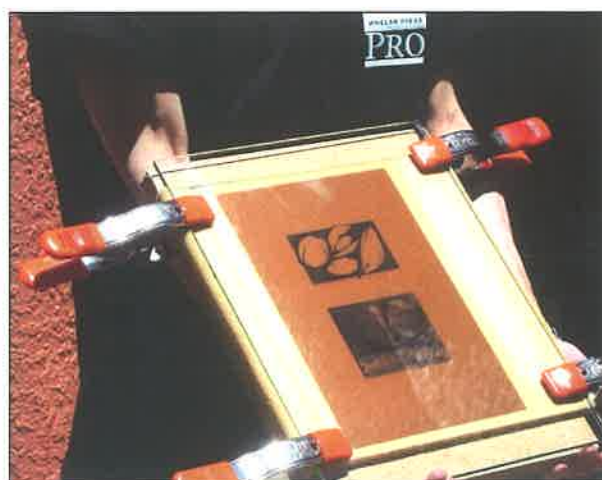
Second exposure 1.5 minutes. Slightly tilt frame from side to side during exposure - this will minimize dust and scratches from showing up in the plate.
