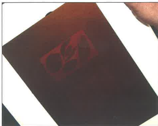
Leave the dry plate on the tray and place it in the sun for 5 to 10 minutes.
