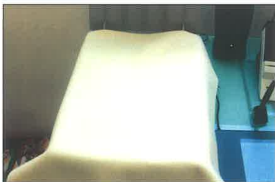
Cover scanner with opaque background. Our felt sizing catcher gives a white neutral background when scanned and drapes well over the objects. Dark colors work well for white objects.
