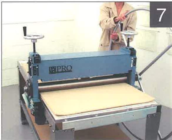
Advance roller by either pushing or pulling hand over hand on drive wheel.
