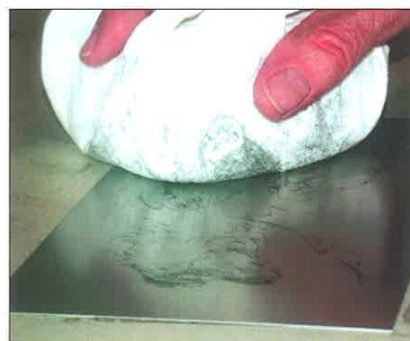
A small amount of image transfer to the cloth is normal. Keep the cloth clean by rotating towel.
