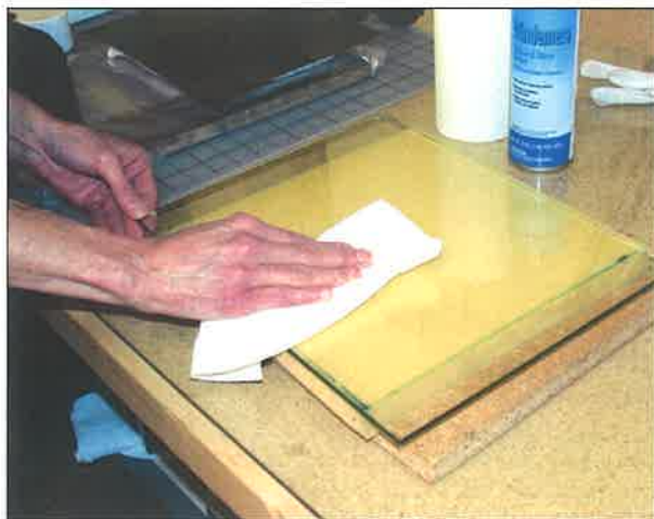
Clean glass surface and inspect for scratches. If a scratch is present locate scratch away from the plate surface.
