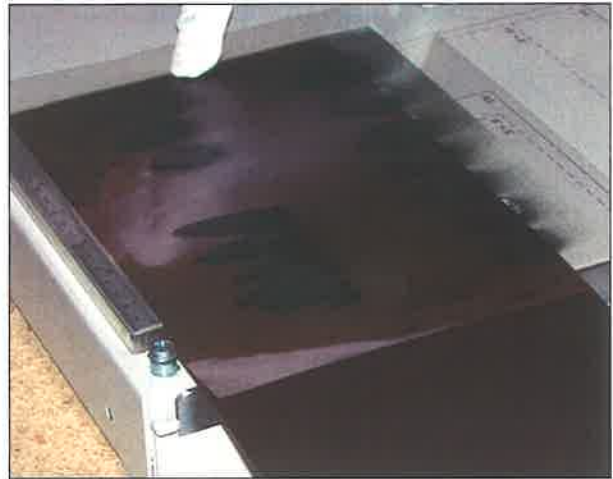
Cut using a heavy paper shear or for best results use the Kuttrimer from Ideal paper trimmers. Cut down through the polymer surface. Wear lint free gloves to keep the plate surface clean and avoid transferring finger prints.
