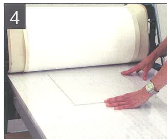
4 Place the plate ink side up and align to the grid.
