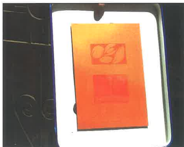
Touch the surface of the plate. If the plate surface feels "smooth" the plate is sufficiently hardened.
