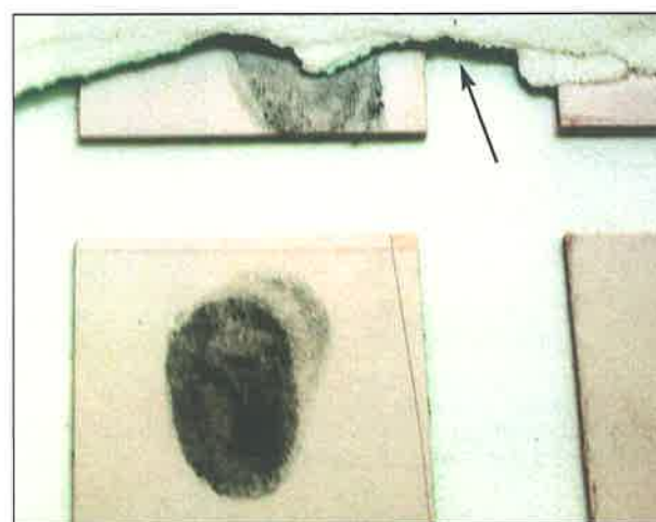
Modeling paste layered over mat chips with graphite finger print.
