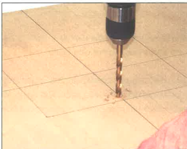
Drill a hole to accommodate the Saber Saw blade.
