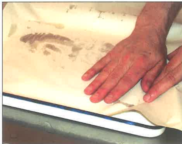
Blot the surface of the plate with newsprint. Be very gentle as the exposed plate has not been hardened.
